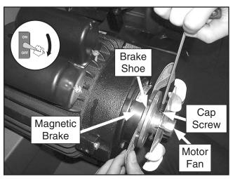
**Figure 16**. Adjusting distance between magnetic brake and brake shoe.
